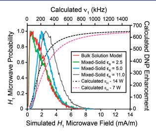
Figure 5. (a) The distribution of calculated  $H_1$  field values for the bulk solution model and mixed solid-solution models from Figure 4b–e. The calculated  $H_1$  values were converted to electron nutation frequencies with eq 3 assuming 14 W of input power ( $\nu_1$ , top axis). The  $H_1$  values were then converted to DNP enhancements with eq 3 and 4 for both 7 and 14 W of input power (right axis, dashed lines).
